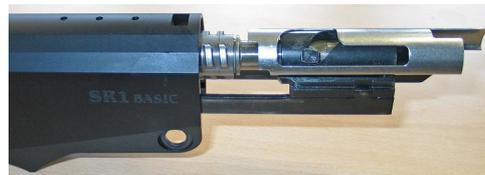
While inserting, the control bolt must be in foremost position.
