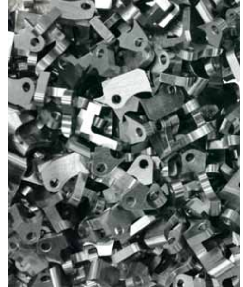
Ejector hammers for side-by-side guns.
