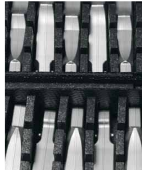
Forging blanks for SR1 housing.
