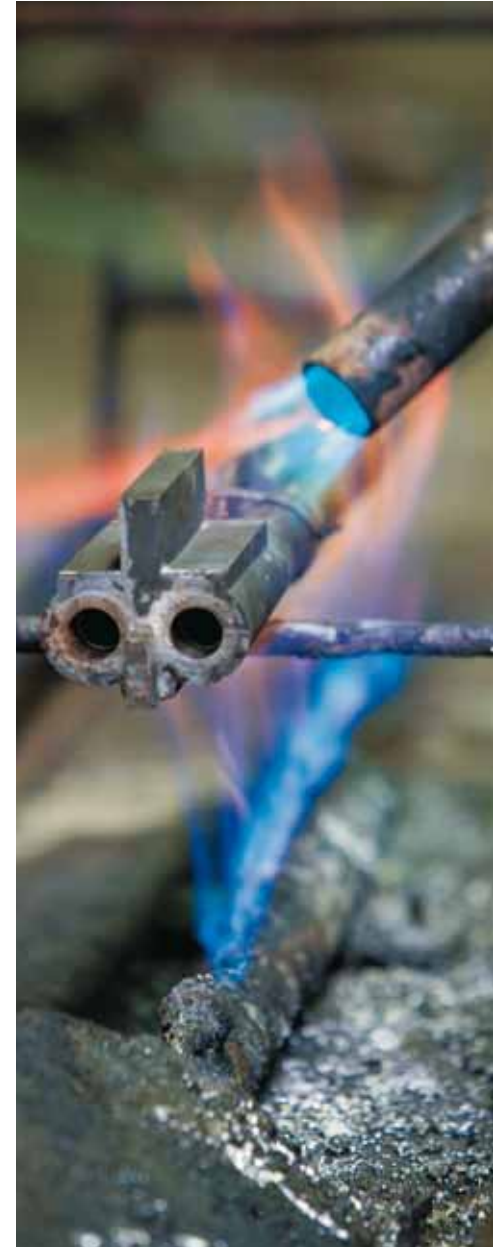
■ Craftsmanship: hand soldered barrels.
