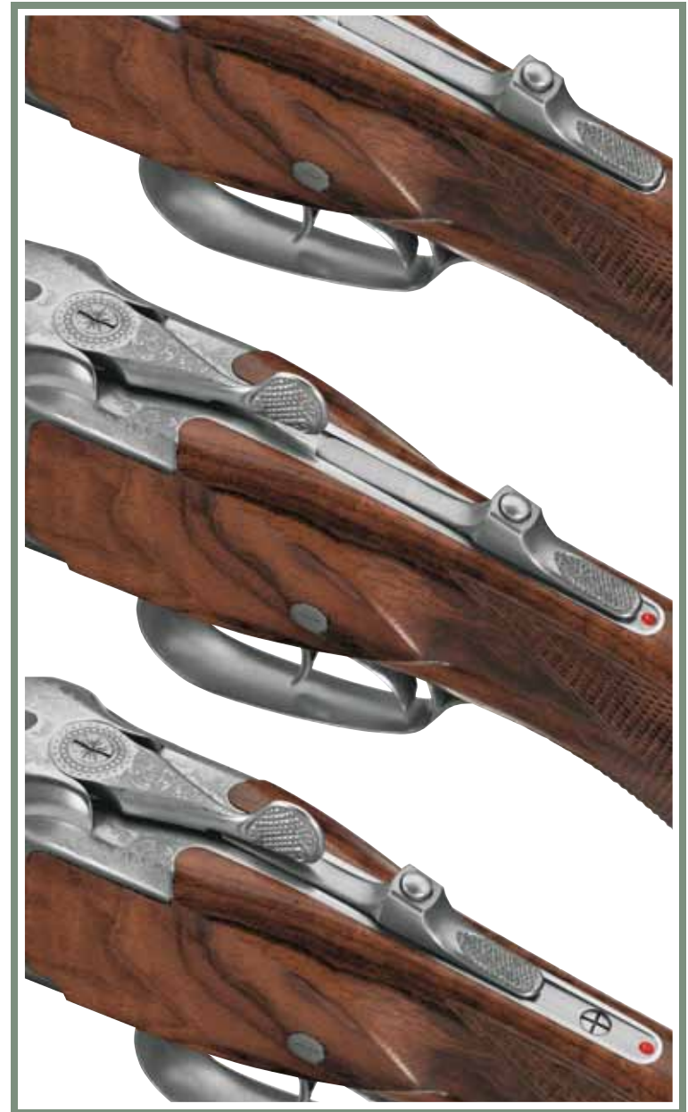
■ Three-position cocking slide: safety and manual cocking system in one.
