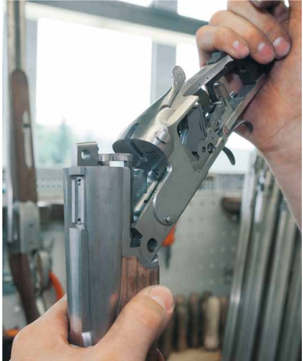
■ The perfect fit: a Drilling action assembled without tolerances.
