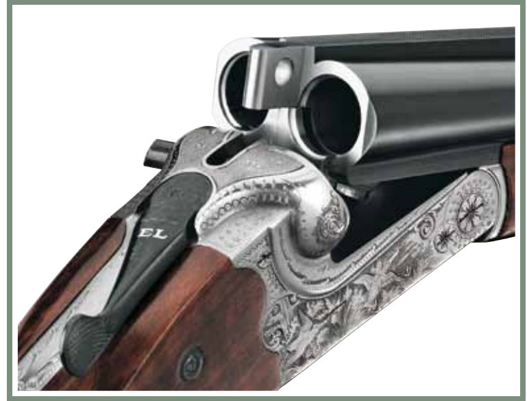
Greener style cross bolt with double bottom bite.
