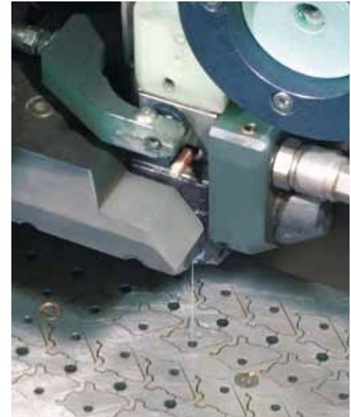
Computer controlled wire-cut EDM.
