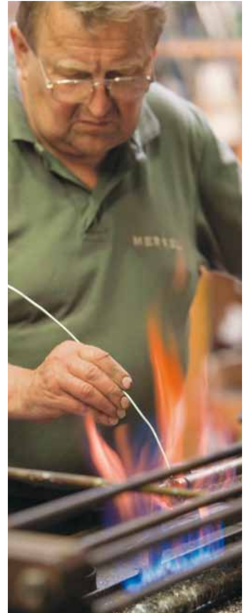
Soft soldering the sight rail.
