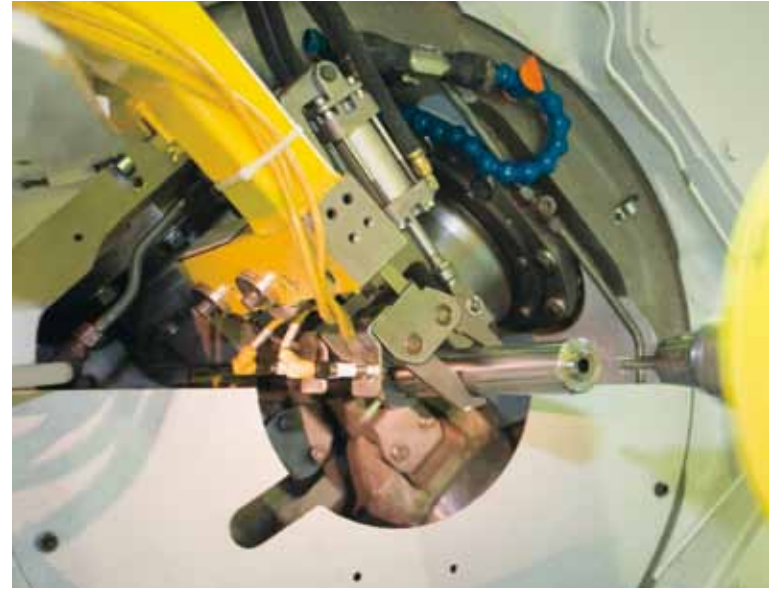
Cold forging with an elemental force hammer mill.
