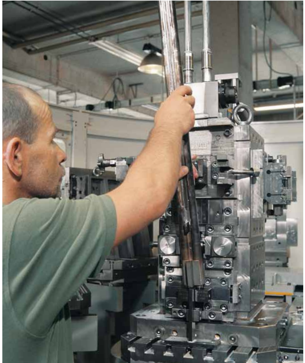
Handwork meets high-tech: the forged barrel is clamped in the CNC milling machine.
