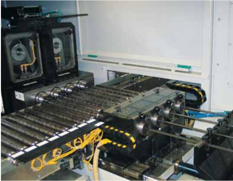
Deep-hole drilling: making a barrel from a steel rod.
